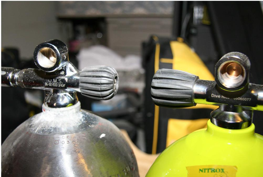
**Figure 3: OMS 300 Bar-DIN and Dive-Rite 200 Bar-DIN Connectors**
